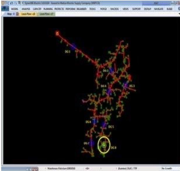
Figure-2: Real time feeders modeling. (a) High loss Feeder Model. (b) Low loss Feeder Model.
