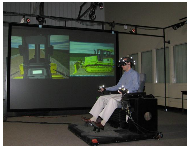
Figure 2: Powerwall system and Hybrid HMD at John Deere (Berg and Vance, 2017).
