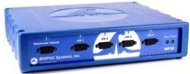
Figure-2: BIOPAC® MP36 Windows Acquisition Unit used for bio potential acquisition. It has three sets of leads i.e. one for reference aka ground (black), one for positive deflection (red) and one for negative (white) as it alternates with the red lead. (courtesy of BIOPAC® MP36 Student Manual)
