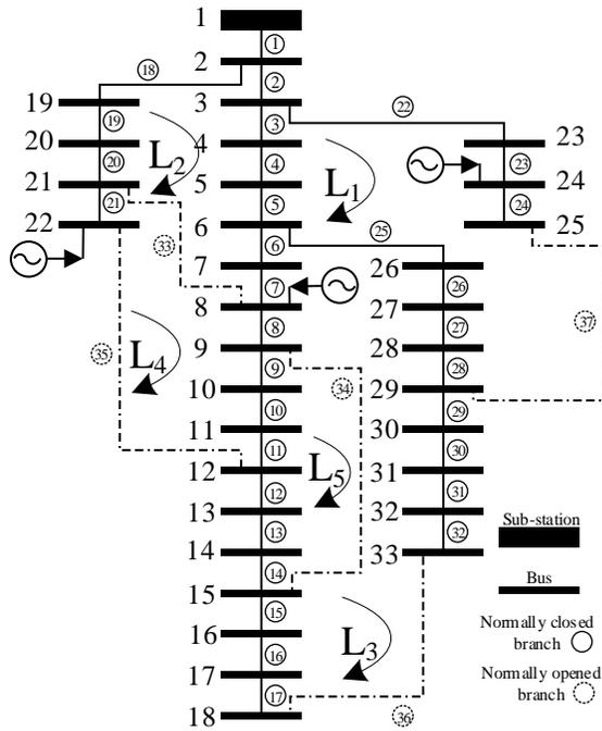
Figure 4. IEEE Standard 33-bus DS reconfiguration and DG integration
