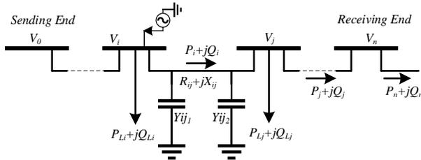
Figure 2. Typical radial DS with DG integration at bus  $i$
