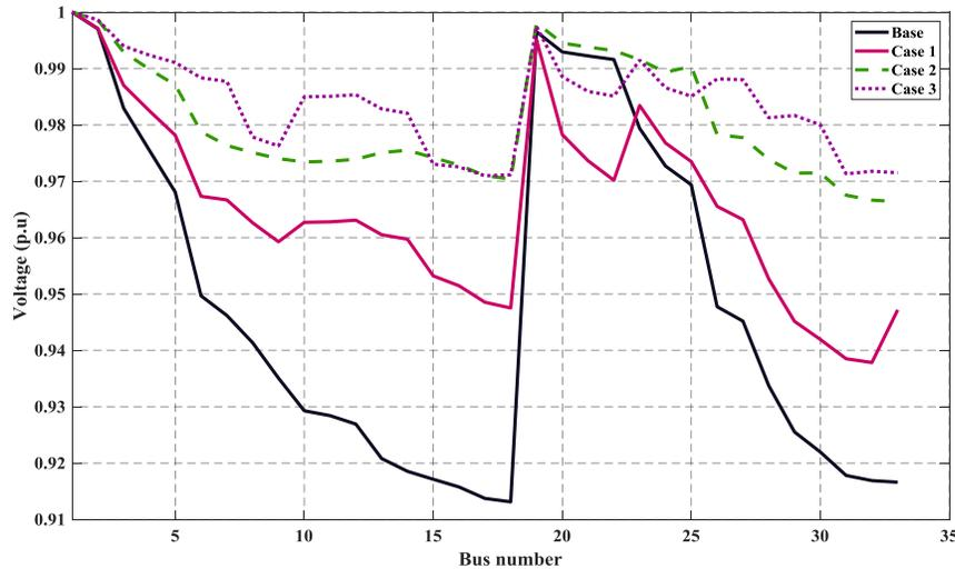
Figure 7. Comparison of voltage level of all cases
