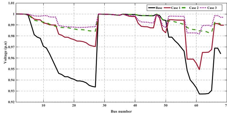
**Figure 9. Comparison of voltage profile between cases 1, 2 and 3 of IEEE 69-bus test system**
