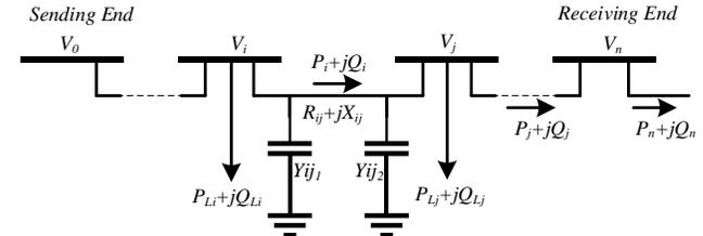
Figure 1. Typical single-line diagram of radial DS
