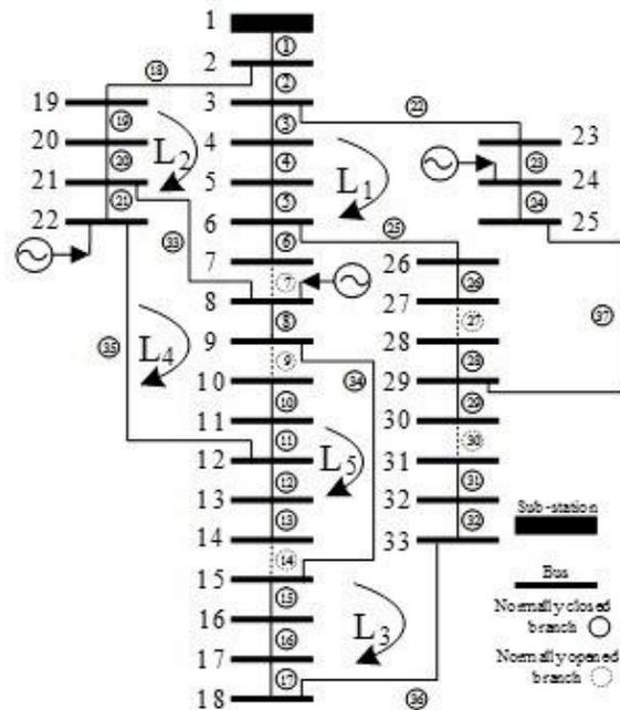
**Figure 6. Final network after the DG integration and reconfiguration**
