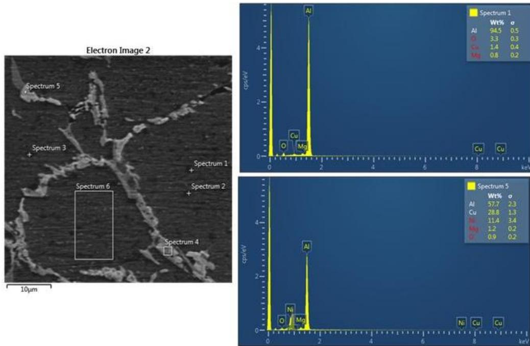
**Figure 8** Microstructure of as cast sample (without any reinforcement) and EDX analysis of spectrum 1 and spectrum 5.
