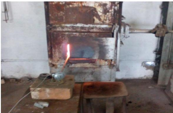
**Figure 2 Gas fired furnace utilized for melting**
