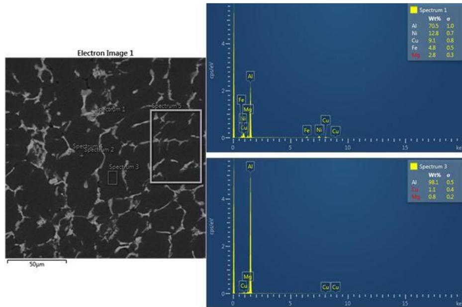
**Figure 9.** Microstructure and EDX analysis of composite sample 5 containing 3wt.% grey cast iron, 2wt.%SiC and 2wt.%Al<sub>2</sub>O<sub>3</sub> particles in 2218 Al alloy.
