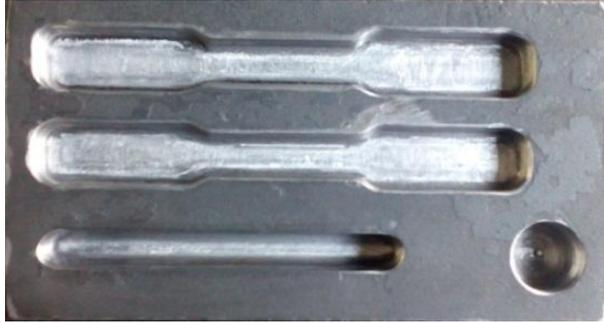
**Figure 1. Mold Die for Casting Composite**
