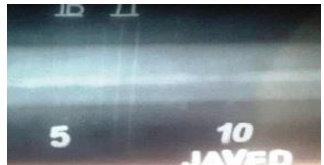
Figure 2 RT report of defect-free Welded joint FCAW-GMAW Process
